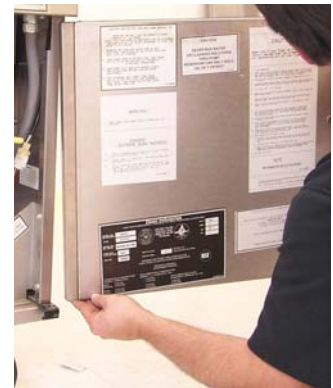
Remove door for easier access to temperature probe.
