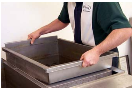
Lift cookpot from rethermalizer.
