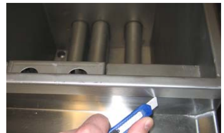
Cut cookpot seal prior to cookpot removal.
